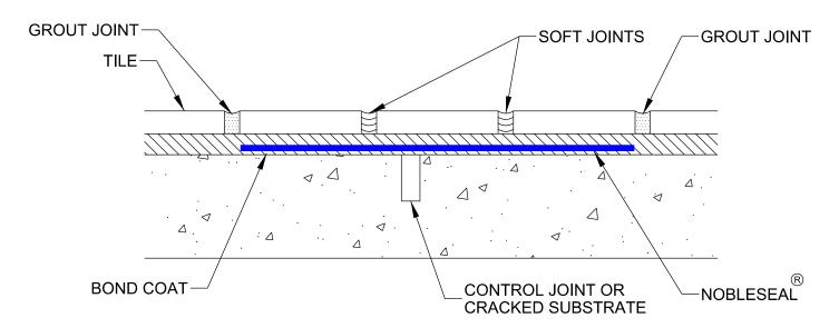
CONTROL JOINTS (CONSTRUCTION, ISOLATION, CONTRACTION)
